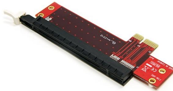
This PCIe x1 to PCIe x16 Slot Extension adapter provides enhanced compatibility between motherboards and a variety of PCI Express expansion cards, allowing you to install a PCIe card (x1 - x16) in an x1 slot.
