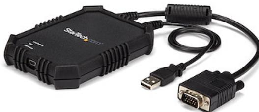
This rugged and portable USB crash cart adapter lets you turn your laptop into a portable console for accessing servers, desktops and laptops, as well as ATMs, kiosks or any computing device that features both VGA and USB ports.
