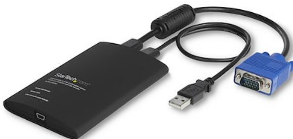
The USB crash cart adapter gives you control of a headless system, turning your laptop into a portable crash cart for rack servers, PCs, ATMs, kiosks, and more.
