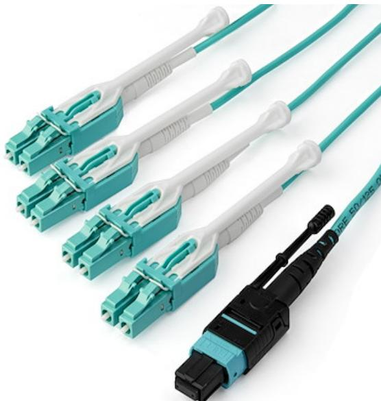
This MPO/MTP to 4x LC breakout cable lets you fan out a single 40Gbps connection from a 40GBase-SR4 QSFP+ transceiver to four 10Gbps LC SFP+ transceivers.
