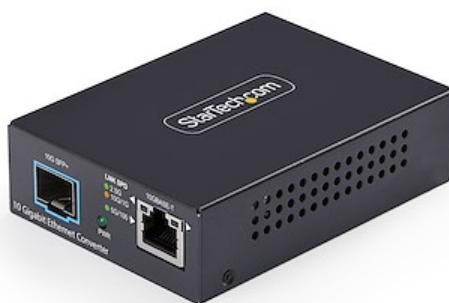
This compact 10G media converter enables seamless copper-to-fiber conversion for network upgrades or long-distance extension. Featuring an open SFP+ slot, it converts 100M to - 10GBASE-T RJ-45 to 10G fiber and supports both multi-mode and single-mode transceivers (10GBASE-SR/LR) for flexible deployment across enterprise and telecom environments.
