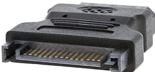
This SATA to LP4 Power Cable Adapter features one LP4 female power connector and a male SATA power connector, allowing you to connect an IDE hard drive to a Serial ATA power connector provided by the computer power supply.
