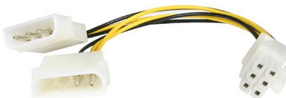
This 6in LP4 to 6 Pin PCI Express Video Card Power Adapter converts a standard LP4 power connector on your existing power supply to a 6 pin PCI Express video card power connector, allowing you to install a PCIe graphics card without having to upgrade the computer power supply.
