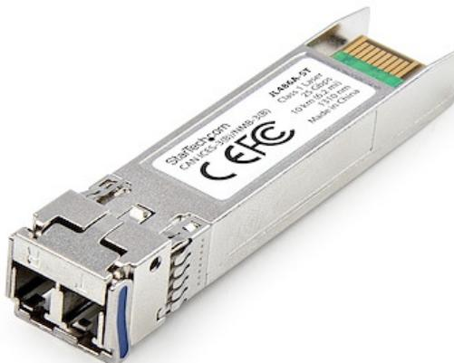
This fiber optic transceiver is the direct equivalent to HPE JL486A for 25Gbps connectivity up to 10km (6.2mi) over LC-terminated Single Mode Fiber (SMF) cable. The optical module has been programmed and tested for seamless integration with HPE switches and routers to ensure compatibility and reliability.
