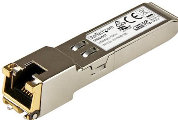
The JD089BST is an HPE JD089B compatible copper transceiver module that has been designed, programmed and tested to work with HPE brand switches and routers. It delivers dependable 1 GbE connectivity over fiber cable, for 1000BASE-T compliant networks, with a maximum distance of up to 100 m (328 ft).
