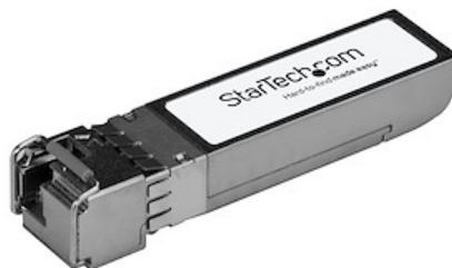
The J9151A-BX-D-ST is an HPE J9151A-BX-D compatible downstream fiber SFP+ transceiver which pairs with StarTech.com's J9151A-BX-U-ST. They are designed, programmed and tested to work with 10GBASE-BX compatible MSA switches and routers. The SFP+ transceiver module supports a maximum distance of up to 10 km (6.2 mi) and delivers dependable 10 GbE connectivity over fiber cabling.
