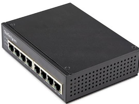
This industrial 8 port gigabit PoE switch features 30W of power and is designed to be installed in harsh environments and supports up to a total of 200W power outputs. Includes hardware for DIN rail or wall mounting.
