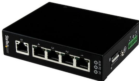
The IES51000 5-Port Industrial Ethernet Switch offers 5 Gigabit Ethernet ports in a compact, IP30-rated metal enclosure, making it the ideal network solution for harsh industrial environments such as factory floors, warehouses or large junction boxes.
