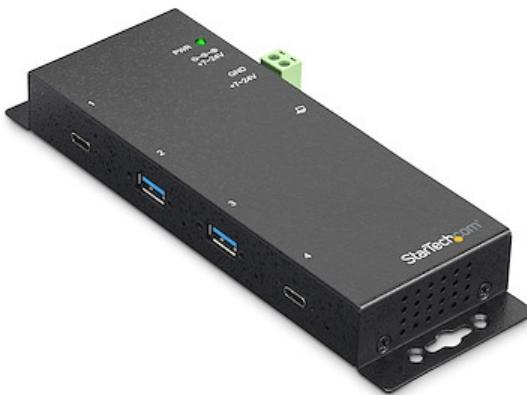
This 4-Port industrial USB hub enables you to connect four SuperSpeed USB 3.2 Gen 2 (10 Gbps) peripherals to your USB-A or USB-C computer. The hub features two USB-A and two USB-C peripheral ports, each with a screw-lock connector, and a metal industrial housing ideal for harsh, industrial environments.
