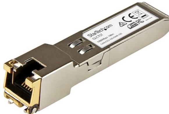
The GLCTST is a Cisco GLC-T compatible copper transceiver module that has been designed, programmed and tested to work with Cisco brand switches and routers. It delivers dependable 1 GbE connectivity over copper cable, for 1000BASE-T compliant networks, with a maximum distance of up to 100 m (328 ft).
