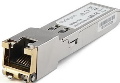
The GLCTEST is a Cisco GLC-TE compatible copper transceiver module that has been designed, programmed and tested to work with Cisco brand switches and routers for extended temperatures. It delivers dependable 1 GbE connectivity over copper cable, for 1000BASE-T compliant networks, with a maximum distance of up to 100 m (328 ft).
