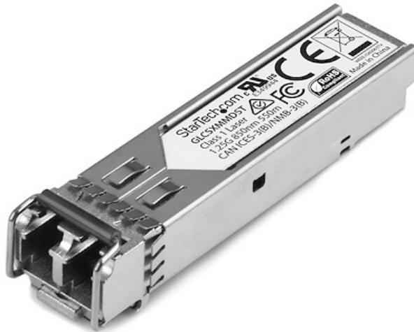
The GLCSXMMST is a Cisco GLC-SX-MMD compatible fiber transceiver module that has been designed, programmed and tested to work with Cisco brand switches and routers. It delivers dependable 1 GbE connectivity over fiber cable, for 1000BASE-SX compliant networks, with a maximum distance of up to 550 m (1804 ft).
