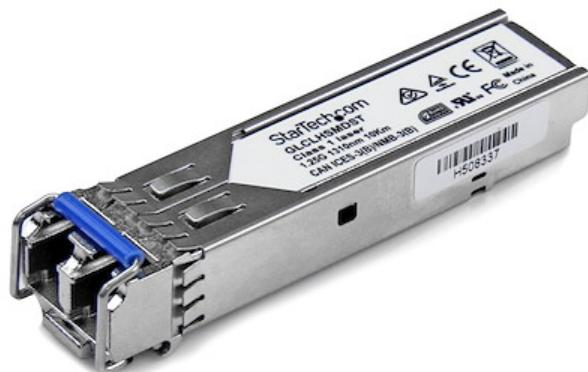
The GLCLHSMDST is a Cisco GLC-LH-SMD compatible fiber transceiver module that has been designed, programmed and tested to work with Cisco brand switches and routers. It delivers dependable 1 GbE connectivity over fiber cable, for 1000BASE-LX/LH compliant networks, with a maximum distance of up to 10 km (6.2 mi).
