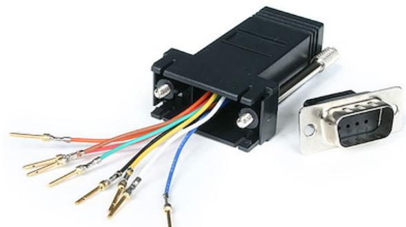
The GC98MF Modular Adapter features a DB9 male connector and an RJ45 female connector. Used for modular RS232, RS422 and RS485 connections, the adapter converts your DB9 female connection into an RJ45 female connection. The adapter allows for custom serial pin out configurations.
