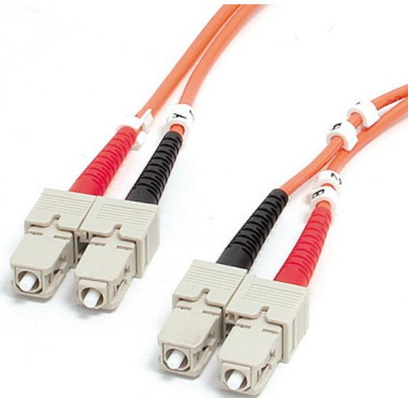
The FIBSCSC2 2-meter (6.6ft) Multimode 62.5/125 Duplex Fiber Patch Cable is terminated at both ends with SC (male) connectors, to provide the necessary connection between fiber networking devices for high-speed, long distance networks.
