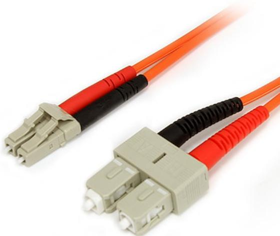
The FIBLCSC5 5-meter (16ft) Multimode 62.5/125 Duplex Fiber Patch Cable is terminated with one LC (male) connector and one SC (male) connector, to provide the necessary connection between fiber networking devices for high-speed, long distance networks.
