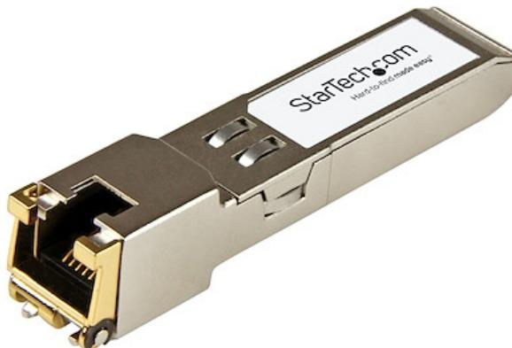
The E1MG-TX-ST is a Brocade E1MG-TX compatible copper transceiver module that has been designed, programmed and tested to work with Brocade brand switches and routers. It delivers dependable 1 GbE connectivity over copper cable, for 10/100/1000BASE-TX compliant networks, with a maximum distance of up to 100 m (328 ft).
