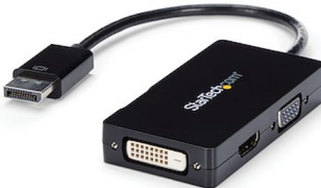
The DP2VGDVHD DisplayPort to VGA, DVI or HDMI converter offers a compact 3-in-1 solution for connecting your DP-equipped desktop, laptop or Ultrabook computer to a VGA, DVI, or HDMI display.
