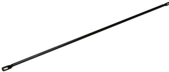
These lacing bars install horizontally on the front or back of your rack to provide a secure mounting point for you to run cables. You can attach your cables to the lacing bars using cable ties to reduce the tension on your cables and prevent damage to the ports on your rack-mount equipment.
