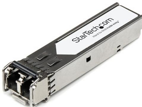
The AR-SFP-1G-SX-ST is an Arista Networks SFP-1G-SX compatible fiber transceiver module that has been designed, programmed and tested to work with Arista Networks brand switches and routers. It delivers dependable 1 GbE connectivity over fiber cable, for 1000BASE-SX compliant networks, with a maximum distance of up to 550 m (1804 ft).
