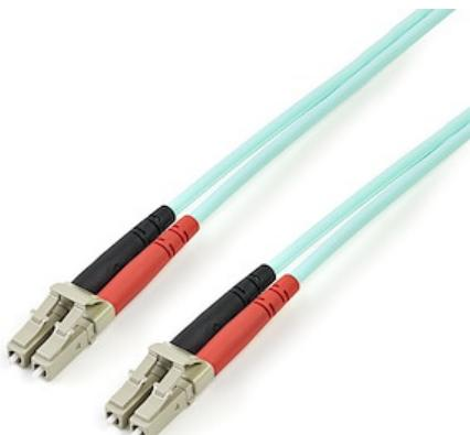
The A50FBLCLC2, 2-meter (6.6ft), 10 Gigabit, Aqua Multimode 50/125 Duplex LSZH Fiber Patch Cable is terminated at both ends with LC (male) connectors and is composed of 50/125 micron OM3 aqua fiber to deliver reliable data transfers at blinding speeds making it perfect for fiber cable runs between multiple backbone switches, hubs and routers as well as higher end networking equipment.
