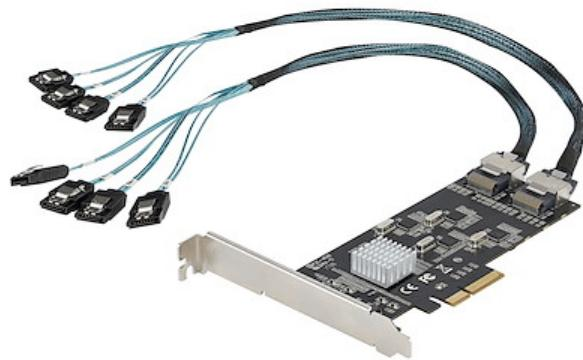
This 8-port SATA III (6Gbps) controller enables you to add eight SATA 6Gbps hard drives (HDDs) or solid State Drives (SSDs) to your computer system or server via an available PCIe x4 card slot. The card supports SATA III and PCI-Express Gen 2 Specifications and four SATA controllers to deliver a high-performance data storage solution.
