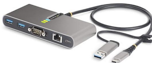
This USB Type-C Hub with RS-232 Serial, Gigabit Ethernet, and 100W USB-C Power Delivery Pass-Through adds two USB 3.2 Gen 1 (5Gbps) Type-A ports to a USB enabled computer. The attached 2ft (60cm) USB-C host cable includes a tethered USB-C to USB-A adapter that enables the USB Hub to easily connect to both USB-A and USB-C host computers.
