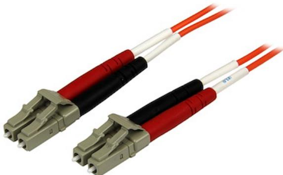
The 50FIBPLCLC3 3m LC to LC Plenum Fiber Cable features 50/125 micron fiber for high-speed, high bandwidth data transmissions over Gigabit Ethernet and Fiber Channel networks, with support for duplex multimode applications.
