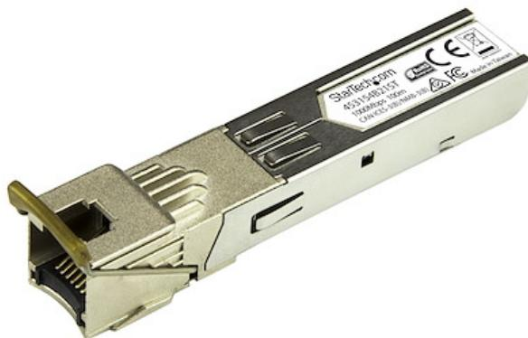
The 453154B21ST is a TAA compliant HPE 453154-B21 compatible copper transceiver module that has been designed, programmed and tested to work with HPE brand switches and routers. It delivers dependable 1 GbE connectivity over copper cable, for 1000BASE-T compliant networks, with a maximum distance of up to 100 m (328 ft).
