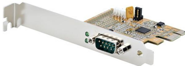
Add serial communication support to your desktop computer or Small Form Factor (SFF) system, using this serial card. RS-232 (DB9) support enables control and communication with a serial peripheral device.
