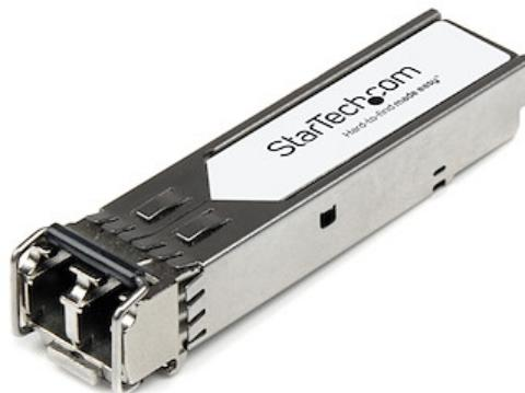
The 10052-ST is an Extreme Networks 10052 compatible fiber transceiver module that has been designed, programmed and tested to work with Extreme Networks brand switches and routers. It delivers dependable 1 GbE connectivity over fiber cable, for 1000BASE-LX compliant networks, with a maximum distance of up to 10 km (6.2 mi).
