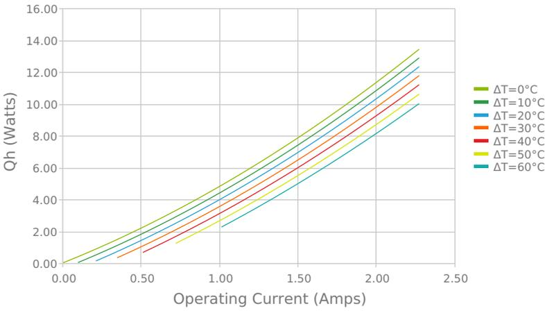
Total Heat Dissipated at Hot Side (Qh=Qc+Pin)
