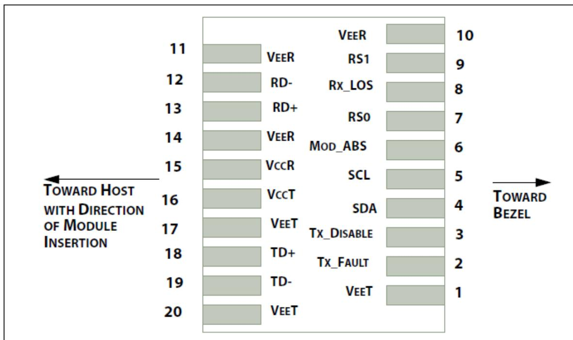
Fiber Optic Transceiver, SFP+, 1550nm, ZR
