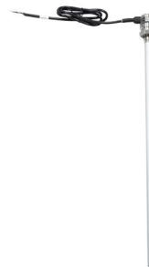
Capacitive liquid level sensor 500mm range, Aluminum sensing rod, 4-20mA, G1/2, direct lead, 1m
