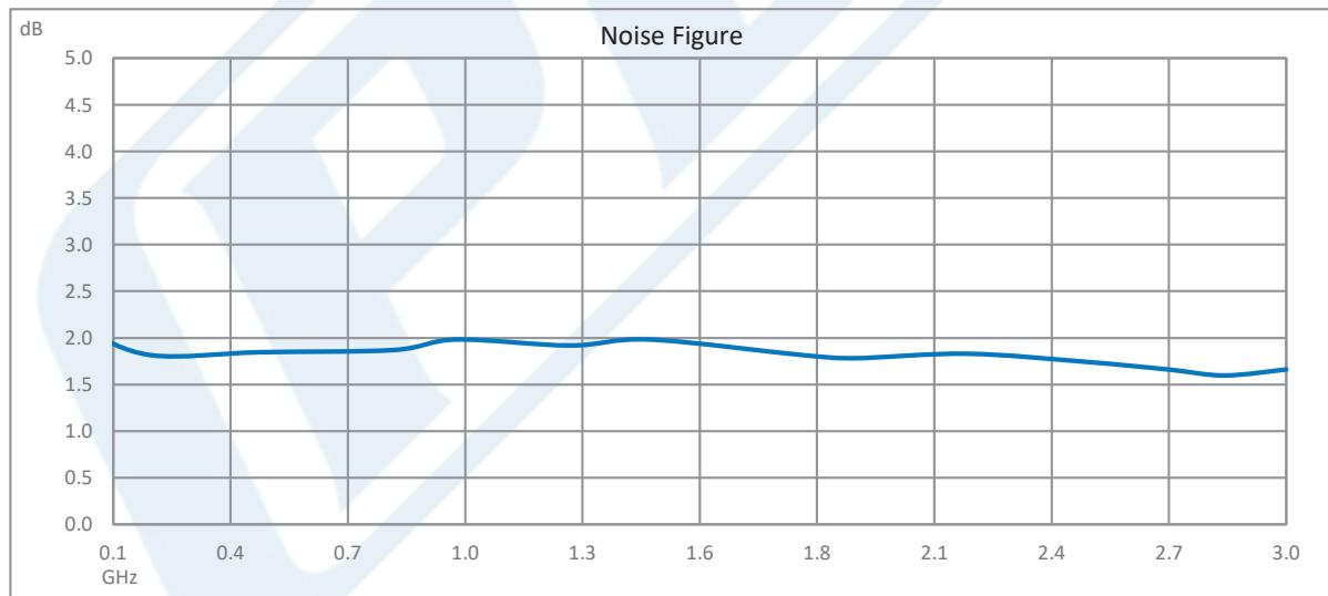
Click the following link (or enter part number in "SEARCH" on website) to obtain additional part information including price, inventory and certifications: [Input Protected Low Noise Amplifier, 30 MHz to 3000 MHz, 1 Watt RF Input Power, 30 dB Gain, 1.7 dB Noise Figure, 12V, SMA PE15A63017](#)
