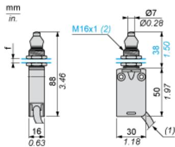
(1) External diameter of cable 7.5 mm.
