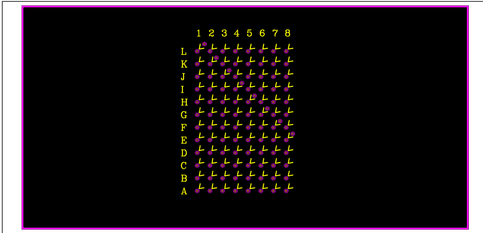
Figure 8 LED Board Component Placement Guide - Top Layer
