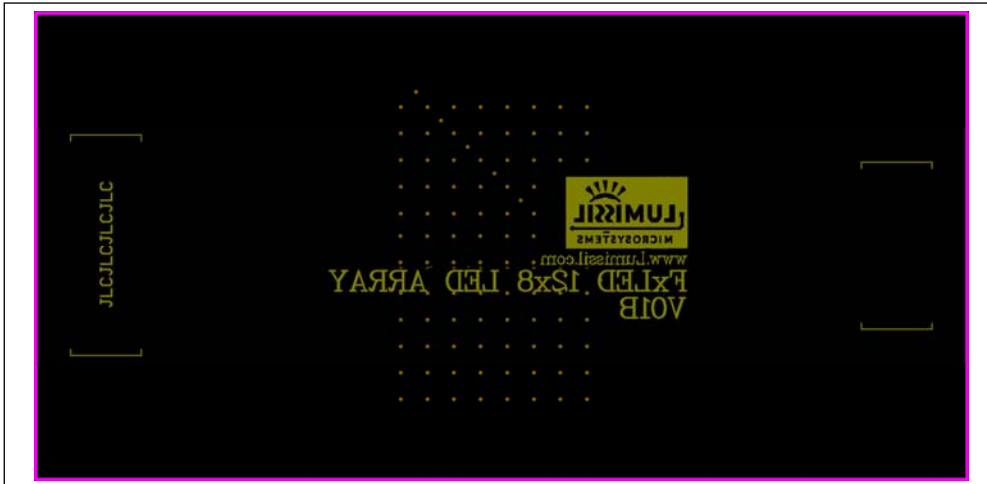
Figure 10 LED Board Component Placement Guide - Bottom Layer
