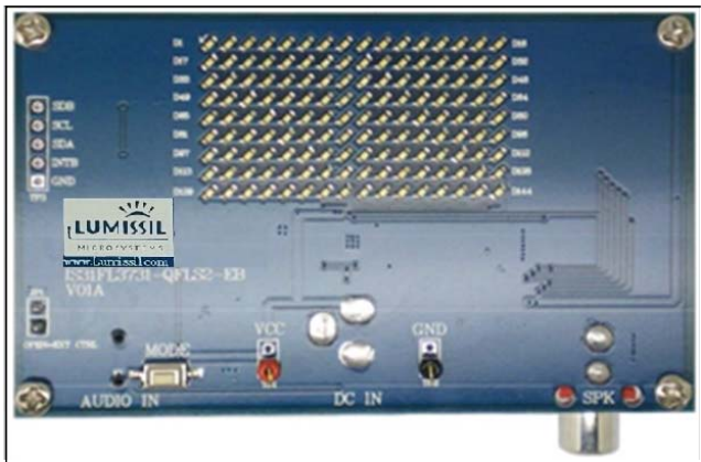
Figure 12 Photo of IS31FL3731 Evaluation Board
