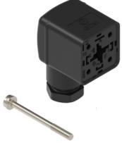
GDM - DIN Valve Connector | Form A | 18mm | #Contacts: 3+Ground | Black Housing PG 9 Thread | No Protective Circuit | 250V
