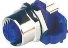
Fast Ethernet Cat5e Data Receptacle Connector: Female, rear mount, M12 - mating side, print contacts - connecting side, 4-pin, D-coded, unshielded, metallic grey housing, 50 V AC / 60 V DC, 4 A
