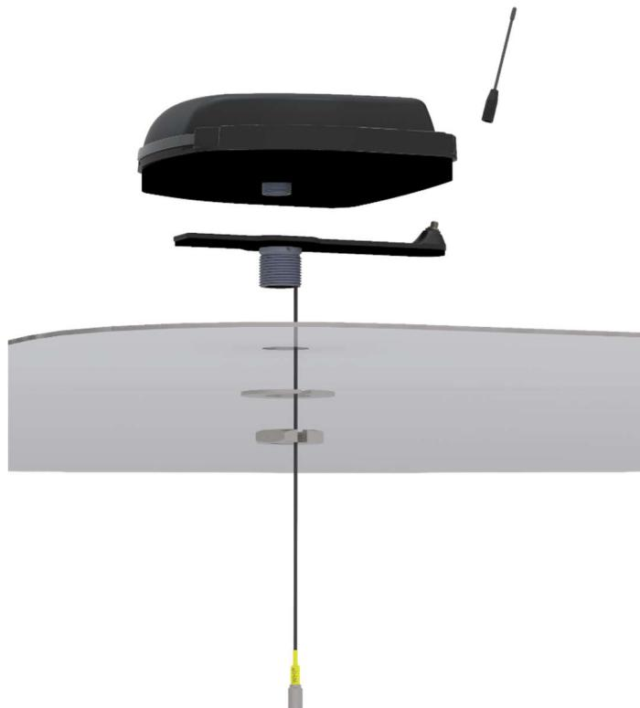
Stack up of installing Whip Base Adapter and whip antenna with AC-Fleet, secured with slotted washer and nut.
