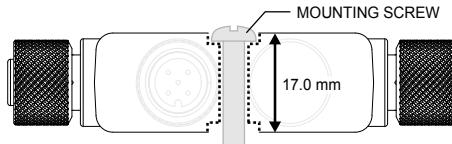
**NOTE:** The dotted line indicates the profile of the counterbore.
