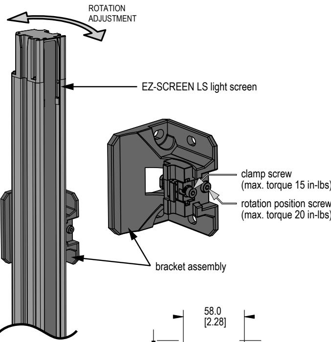
2 Slide inner bracket assembly into outer bracket groove.
