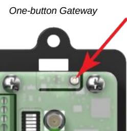
The LEDs flash alternately when the Gateway is in binding mode. Any Node entering binding mode will bind to this Gateway.
