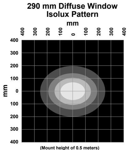
Lux and irradiance values shown are typical at 25 °C and with clear windows; light intensity lowered by 40% on diffuse window models.
