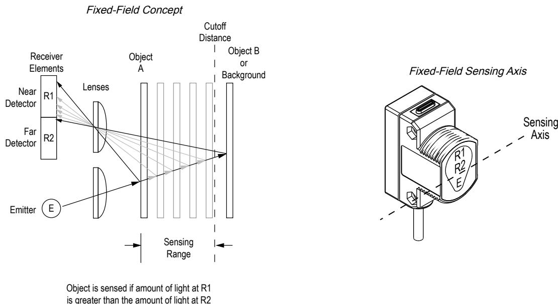
In the drawings and information provided in this document, the letters E, R1, and R2 identify how the sensor's three optical elements (Emitter "E", Near Detector "R1", and Far Detector "R2") line up across the face of the sensor. The location of these elements defines the sensing axis, see "["Figure: Fixed-Field Sensing Axis" on page 7](#)".
