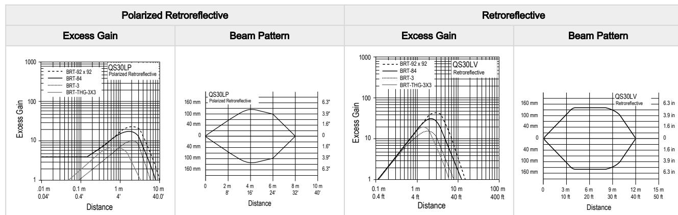
Fixed field performance is based on using a 90% reflectance white test card.
