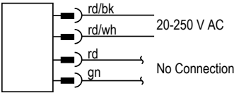
4-pin 1/2 in-20UNF (1/2-in Dual Key) quick disconnect emitters
