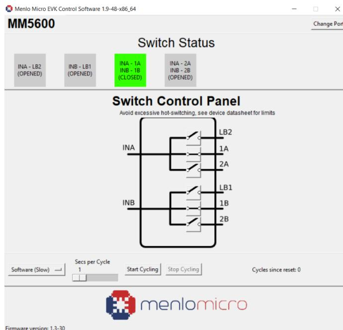
7. To connect the input ports (INA and INB) to the output ports (2A and 2B), click on either “INA\_1A” switch or “INB-1B” switch, then both switches are on/off together.
