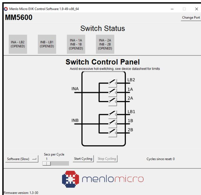
6. To connect the input ports (INA and INB) to the output ports (1A and 1B), click on either “INA\_1A” switch or “INB-1B” switch, then both switches are on/off together.
