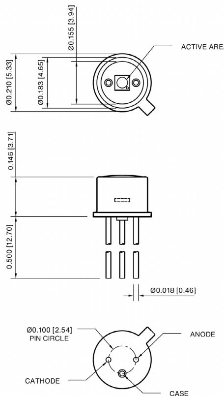
Note: Lead soldering temperature (1/16 inches from case) 260°C for 3 sec.
