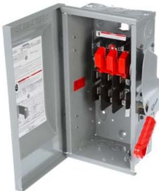
Siemens Low Voltage Circuit Protection Heavy Duty Safety Switch. 3-Pole 3-Fuse and solid neutral Fused in a type 1 enclosure (indoor). Rated 240VAC (30A).
